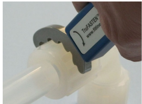
Fig. 17 Finish tightening with torque wrench.
