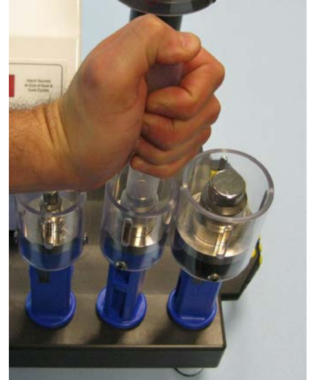
Fig. 9. Push tube onto flaring mandrel
