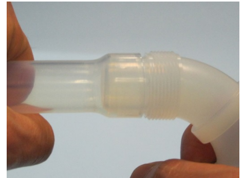
Fig. 15 Flared end of tube must be pushed up to flared end of fitting.
